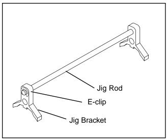
Figure 8. Knife setting jig components.
